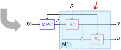
• MPC designed to handle input/output constraints and improve performance
